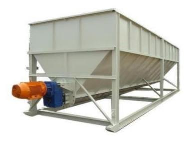
• Pallet Conditioner: This machine is used for moisturizing the material with Steam.
